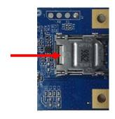
**Step 3: Insert SIM**Insert the SIM card to the SIM holder.
