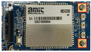
Step 4: Connecting antenna cables accordingly.
