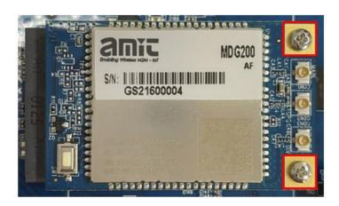
Step 4: Connecting antenna cables accordingly.
