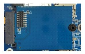
\*If the host board is designed for a M.2 3052 module, please use the screw hole as marked below.
